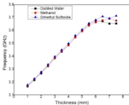
Figure 7. Resonant frequency at different thickness
