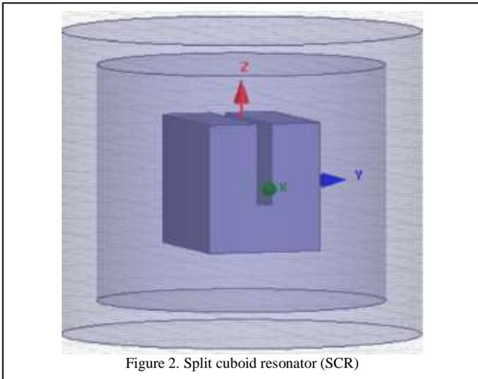
Figure 2. Split cuboid resonator (SCR)
