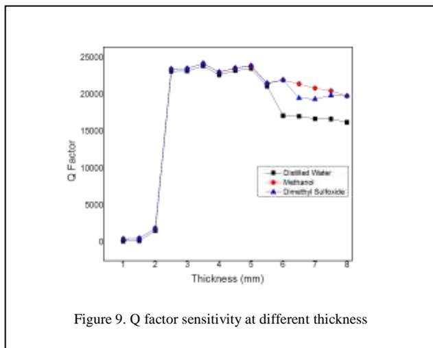
Figure 9. Q factor sensitivity at different thickness
