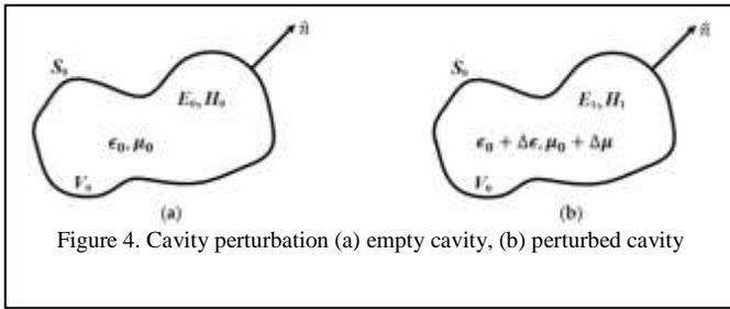
Figure 4. Cavity perturbation (a) empty cavity, (b) perturbed cavity
