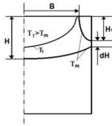
Figure 2. a) The temperature distribution at EBM in Cu ingot cross-section at input electron beam power 22 kW, radius of the beam 15 mm and crystallization speed 3 mm/min, b) Molten pool geometry parameters.
