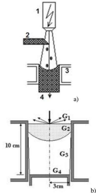
Figure 1. Electron beam drip melting a) 1 – electron gun, 2- feeding rod, 3 – water cooled crucible, 4 – ingot, b) geometrical conditions and boundary conditions:  $G_1$  – top ingot surface,  $G_2$  – interface molten pool/crucible,  $G_3$  – free side ingot surface,  $G_4$  – interface – ingot/puller.
