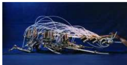
Figure 1. Robot III, hexapod modeled based on the structure and function of a cockroach.
