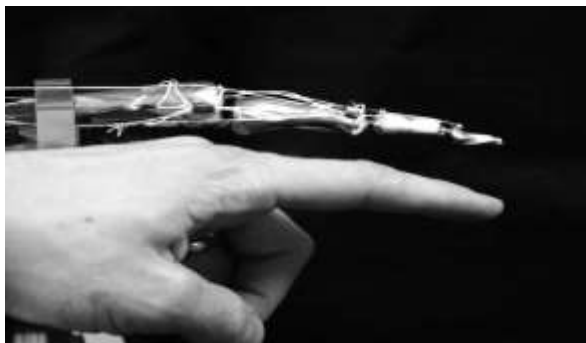
Figure 2. Anatomically Correct Testbed (ACT) index finger. From Neurobionics Laboratory
