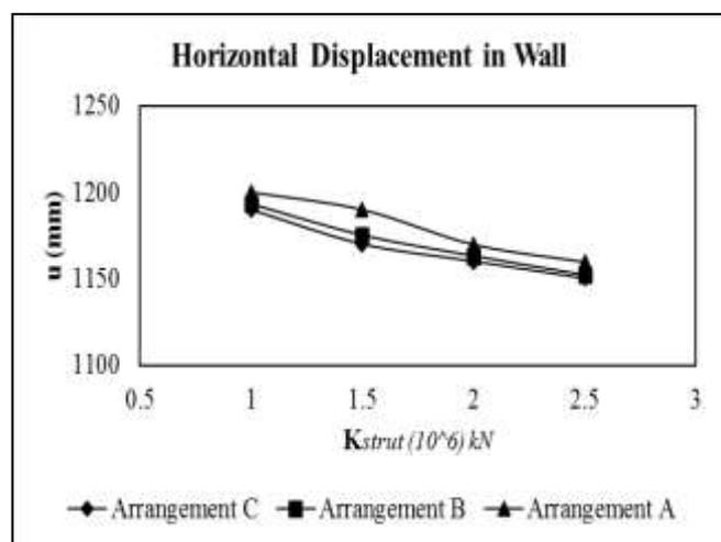
Figure 3: Effect of  $K_{strut}$  on horizontal displacement of diaphragm wall
