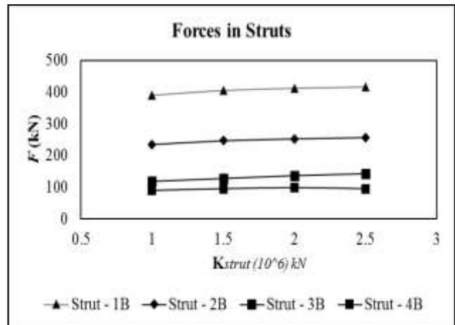
Figure 7: Forces in Strut for arrangement B
