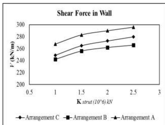
Figure 4: Variation in Shear force in diaphragm wall with varying  $K_{strut}$
