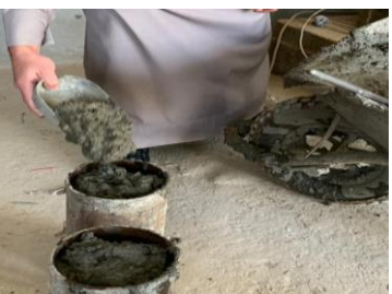
D) The casted concrete specimens are cured for 28 days
