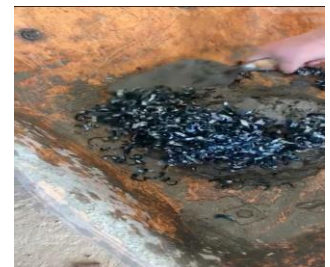
B) The steel fibers are added to the plain concrete
