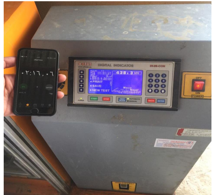
B) Plain concrete (1% added waste steel fiber)
