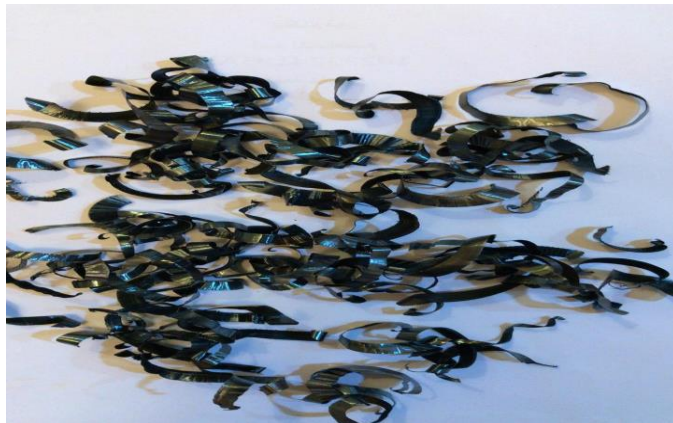
Figure 3: The hooked-end industrial steel solid wastes.
