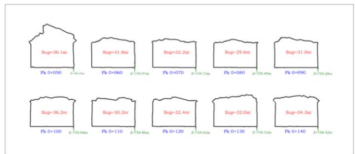
Figure 4.- Cross-sections each 10 m.
