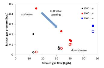
Figure 4. Gas pressure upstream (solid symbols) and downstream (hollow symbols) of the EGR module
