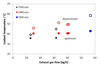
Figure 3. Gas (top) and coolant (bottom) temperature upstream (solid symbols) and downstream (hollow symbols) of the EGR module
