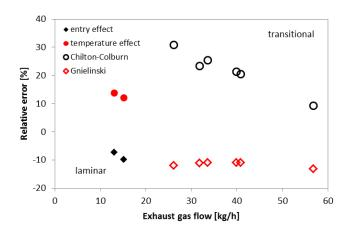
Figure 8. Relative error of empirical correlations from the literature with respect to heat transfer coefficient calculated based on experimental data
