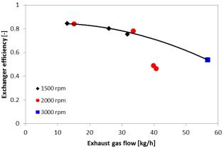
Figure 5. Effectiveness (top) and efficiency (bottom) calculated in the studied exhaust gas flow range
