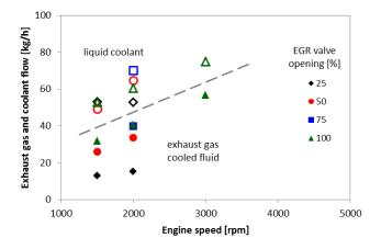
Figure 2. Flow values on the gas (solid symbols) and liquid (hollow symbols) sides
