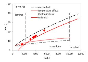
Figure 7. Correlation between *Nu* and *Re* numbers; data from the current experiment are represented with points, laminar equations are illustrated with double lines, while transitional-turbulent correlations with solid lines
