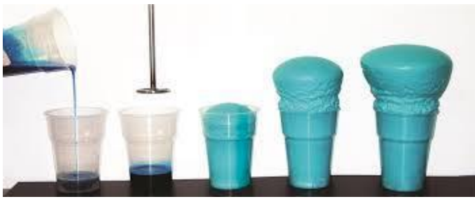
Figure 2: The steps of preparing the polyurethane compounds.
