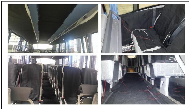
Figure 4. Heating surfaces applied in to test vehicle
