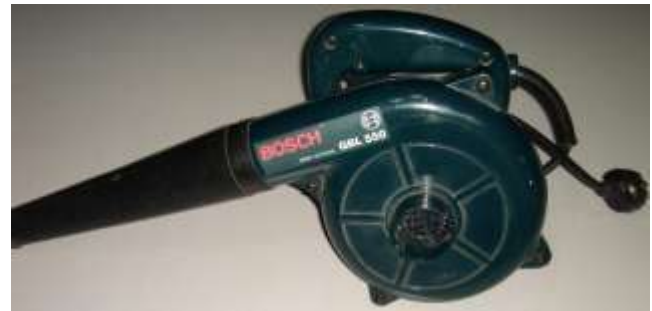
Figure 6. The blower used to clean the dust.
