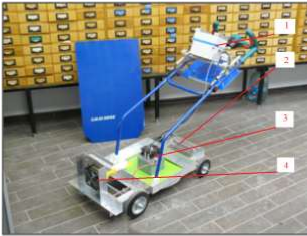
Figure 9. Picture of the detector system on the wheeled platform: 1) control unit; 2) the battery; 3) the detection unit; 4) additional fan.
