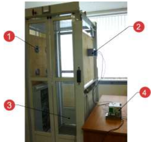
Figure 12. Picture of experimental unit of portal radiation monitor: 1 – group fans; 2 – detector; 3 – doors; 4 – control and processing block.
