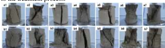
Figure8. The development of the studied samples behavior from ductile (for untreated compacted samples) to brittle (for stabilized samples); a) EB; a1) Natural Compacted EB; a2) EB+CKD 7days; a3) EB+CKD 28days; a4) EB+CKD 90days; a5) EB+L/CKD 7days; a6) EB+L/CKD 28days; a7) EB+L/CKD 90days; b) EQ; d1) Natural Compacted EQ; b2) EQ +CKD 7days; b3) EQ +CKD 28days; b4) EQ +CKD 90days; b5) EQ +L/CK 7days; b6) EQ +L/CKD 28days; b7) EQ +L/CKD 90days
