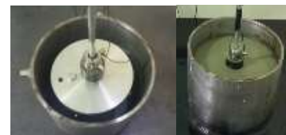
Figure 4. Experimental arrangement of scale drilling apparatus with and without drilling mud
