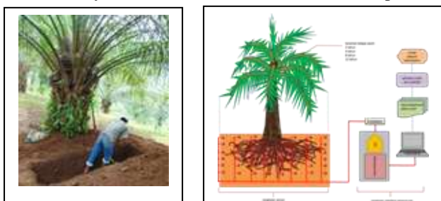
Figure 12. Soil hole for a multichannel system tested and measurement scheme
