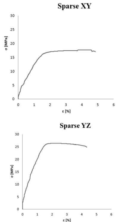
Figure 9. Average tensile strength - sparse XY and YZ.
