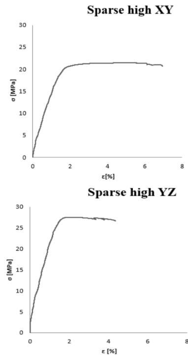
Figure 8. Average tensile strength - sparse high XY YZ.
