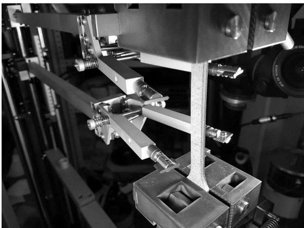
Figure 6. Tensile strength test on 3D printed specimens.
