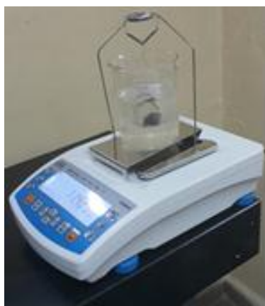
Figure 3. The density measurement of the friction composites
