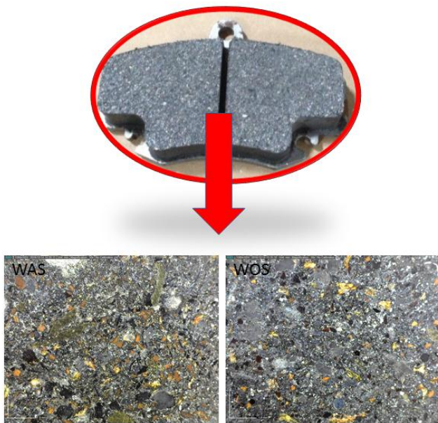
Figure 4. Optical micrographs of the brake friction composites
