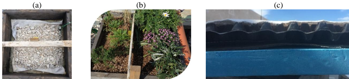
Figure 1: (a) TGBR (b) EGR16 mockups and (c) different intermediate layers installed on the chemical engineering building
