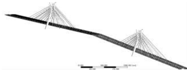
Figure 3.4. Side View of discretized Lekki Bridge
