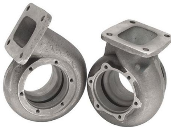
Figure 1 - Image of turbocharger turbine volute casing
