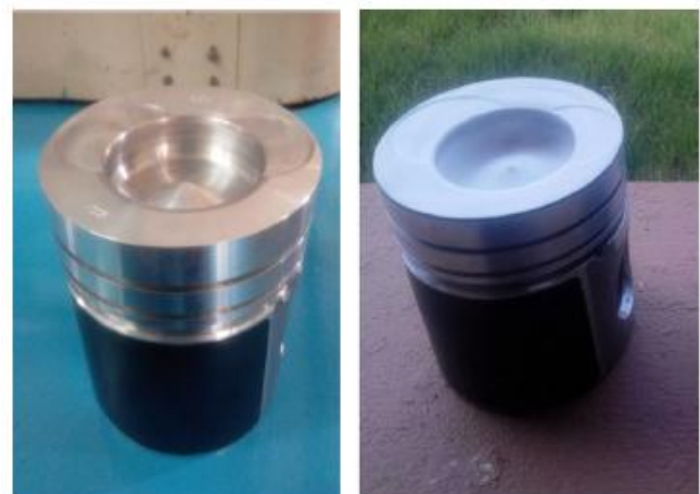
Figure 2 - Snapshots of uncoated baseline engine piston (left) and YSZ coated piston (right). (Sivakumar and Senthil Kumar 2014).
