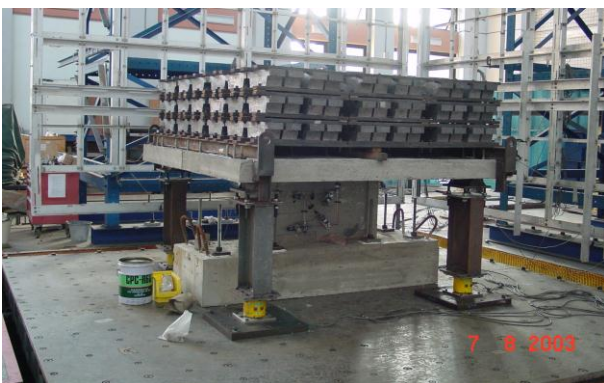
Figure 2. Test set-up of shake table tests
