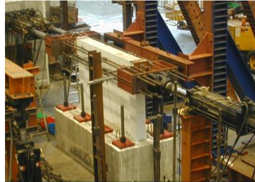
Figure 5. Set-up of reversed cyclic tests
