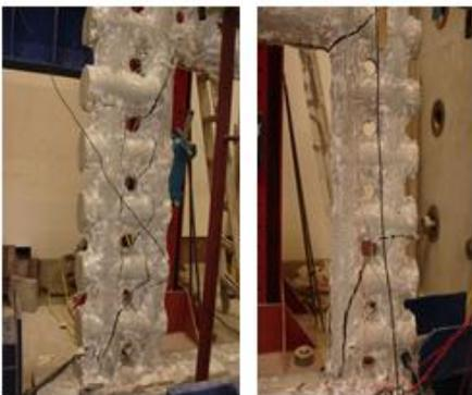
**Figure 7 SD1 after applying monotonic load**
