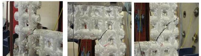
Figure 4 Cracking of SW1, lower left corner (left), upper top corner (center), lower right corner (right)
