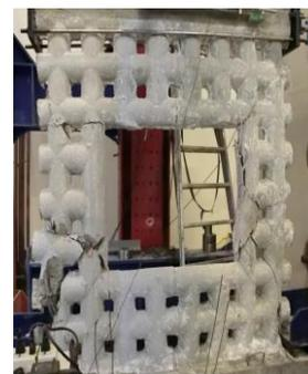
Figure 5 SW2 after cyclic loading
