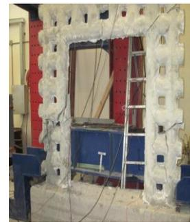
**Figure 11 SD2 after applying cyclic load**
