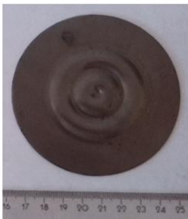
Figure 4. Part obtained by One-channel sheet hydroforming
