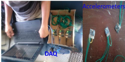
Figure 4.0 Accelerometers and the DAQ
