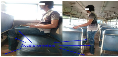
Figure 3.0 Placement of accelerometers under sitting and standing orientations of the passenger
