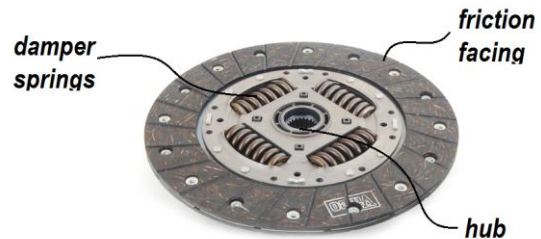
Figure 2. Clutch disc components (Valeo Automotive)
