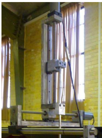
Figure 2. The probe transmission mechanism
