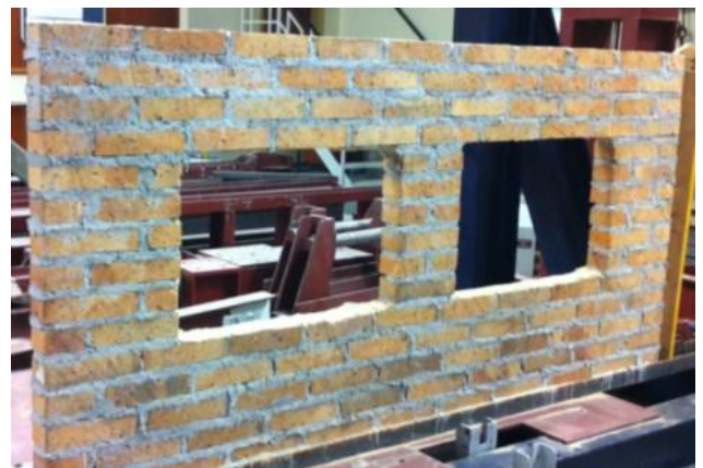
Figure 1d Wall with 30% opening
