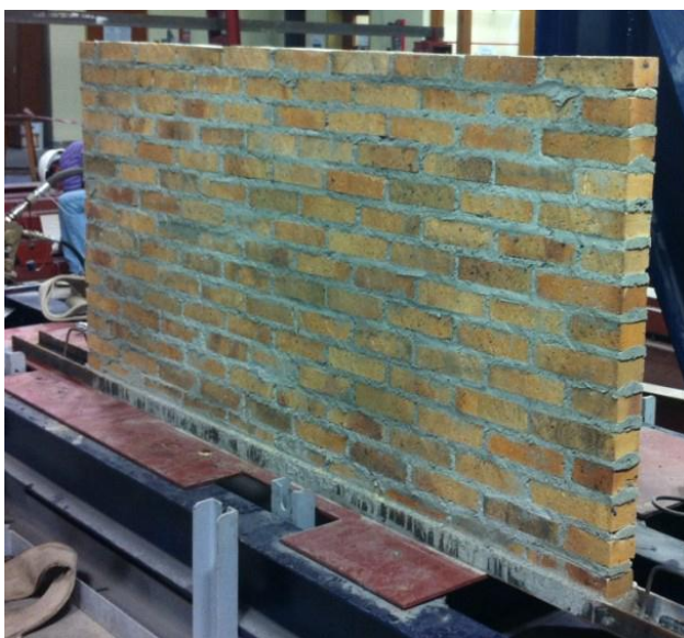
Figure 1a Wall without opening
