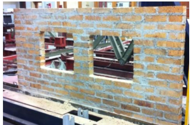
Figure 1c Wall with 20% opening
