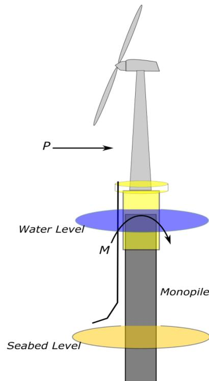
Fig. 1 Loads acting on Offshore Wind Turbine Structure.
