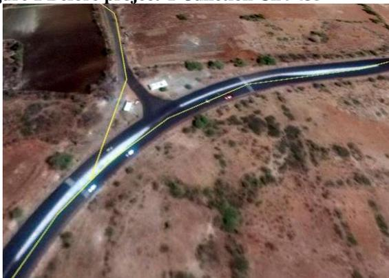
Figure 2 After project T-Junction with right turning lane Ch 9435
