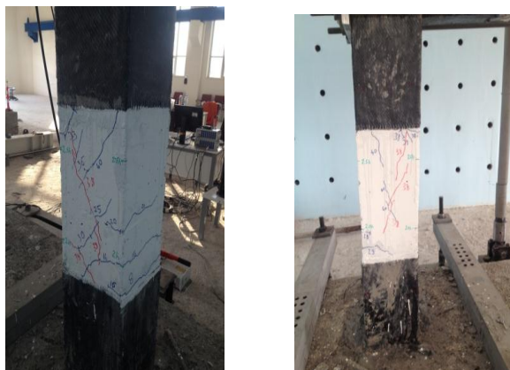
Fig. 10: CBFS-DC Specimen's Crack Development
