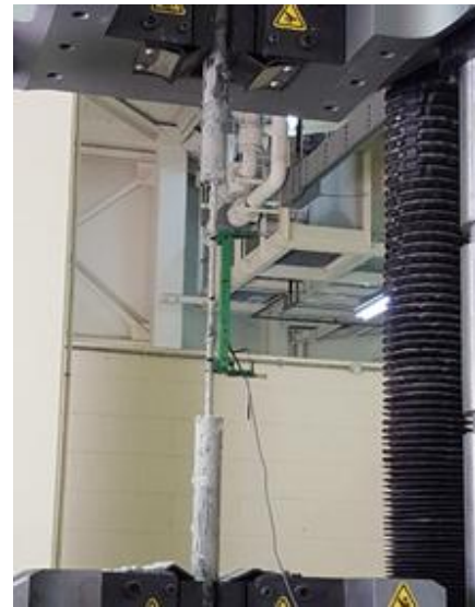
Figure 2. FRP Reinforcing Bar under Tensile Strength Test.
