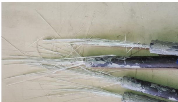
Figure 4: GFRP Reinforcing Bars after Failure.
