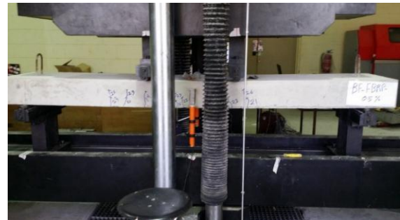
Figure 6 One-Way Concrete Slab during Flexural Test.
