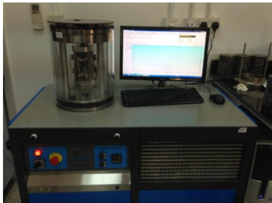
Figure 5. AMPT system for dynamic modulus test
