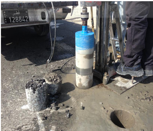
Figure 1. Extraction of field cores from the test sections
