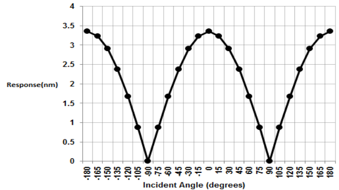
Fig. 9. Displacement with respect to change in Incident Angle
