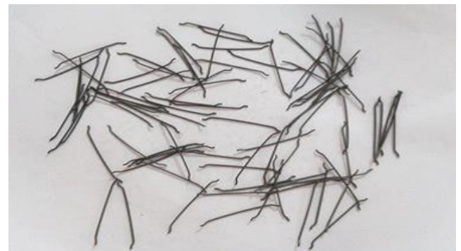
Figure 3. Hooked end steel fibres of aspect ratio 50
