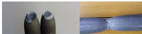
Figure 15. Traction test of a steel bar
