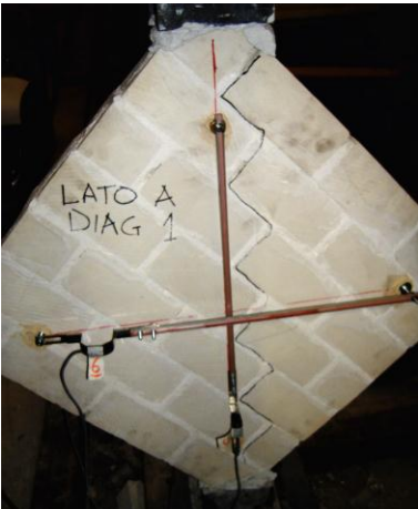
Figure 15. Cracks after diagonal test
