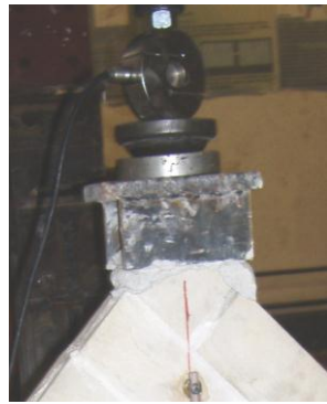
Figure 10. Load cell ball joint
