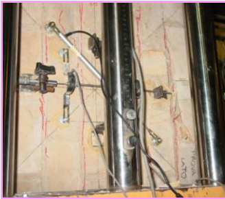
Figure 13. Cracks after compression test x direction
