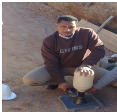
Fig. (4): Sand cone method in the Field, after Mahmoud.M.Abuzei
