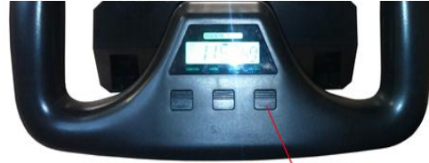
Fig. 16 Flight Yoke used in operator station to control robot.
