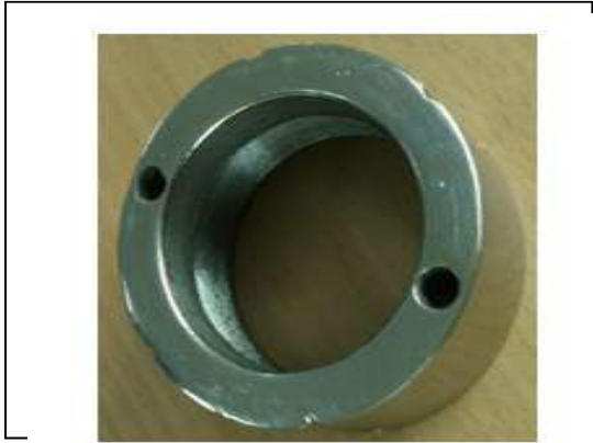
Fig.2: Clamp Sleeve which is located inside the crimping head and outside the inside the crimping head and outside the crimping tong
