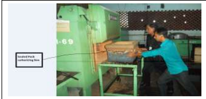
Fig. 6: Pack carburizing Box inserted to the Furnace
