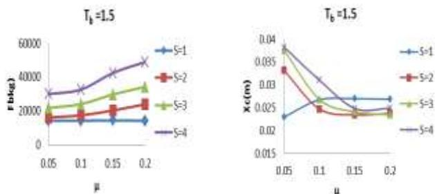
Figure 12. The variation of resisting force of the isolation system w.r.t friction coefficient
