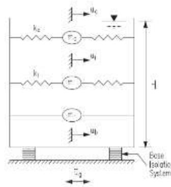
Figure 1. Three-degree of freedom of liquid storage tank
