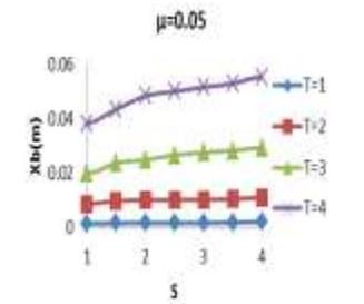
Figure 10. The variation of displacement of bearings relative to the ground w.r.t slender ratio of tank
