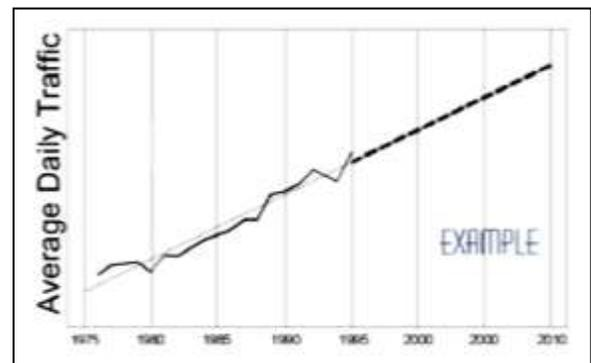
Figure 2. Graphical Method of Traffic Forecasting
