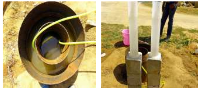
Fig. 2. Experimental setup for Double ring infiltrometer
