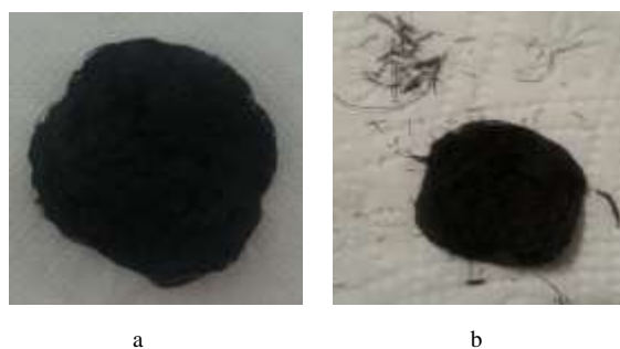
Figure 3. The a) pre-adsorption and b) after desorption images of nonwoven surfaces obtained from coagulation in pH 7 NaOH containing coagulation bath
