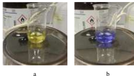
Figure 4. The gas washing solutions a) before titration b) after titration
