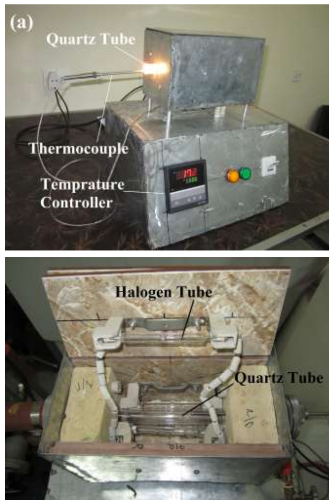
Figure 1. The camera images of the Halogen tube furnace (a) Halogen tube furnace with temperature controller during oxidation of zinc (b) Inner view of the halogen tube furnace.
