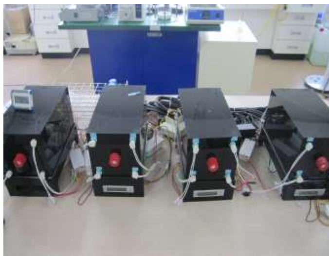
Figure 1. Pictorial view of the batch photocatalytic reactor (from right to left: 1. only UV, 2. uncoated EPP balls with UV, 3. TiO 2 -coated EPP balls with UV, 4. only TiO 2 -coated EPP balls without UV)
