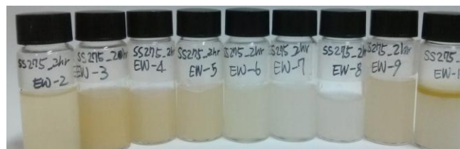
Figure 3. Extraction water of contaminated soil D (collect samples in every 10mins after 40min).
