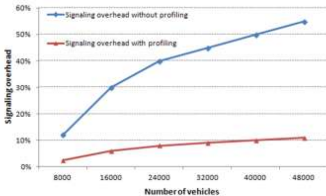
Figure 3. Signaling overhead in function vehicles number
