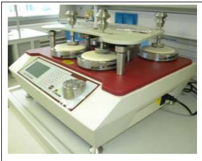
Figure 1. 4 Head Martindale Abrasion Tester
