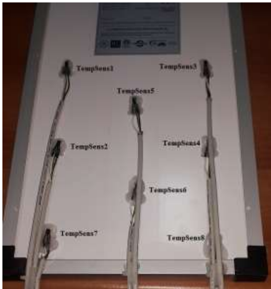
Figure 1. Back side of PV module and positions of the sensors
