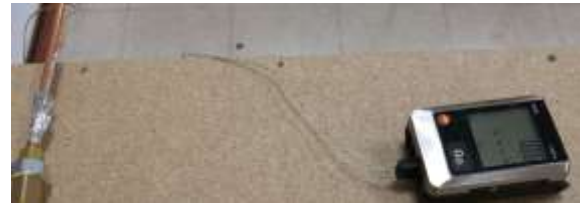
Figure 3. Temperature data logger
