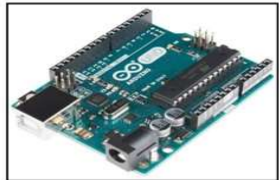
Figure 3. Arduino Uno R3 Microcontroller
